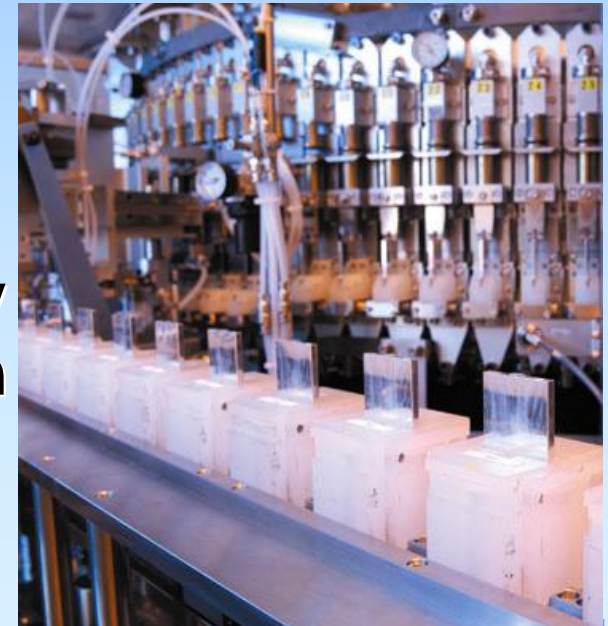
Production line for lithium-ion batteries 17
